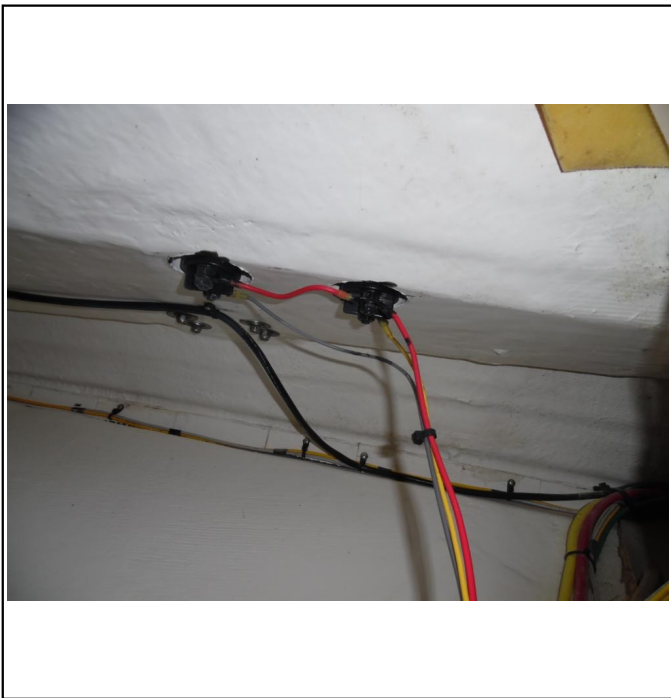
Windlass - Unsupported Wiring in Anchor Locker
