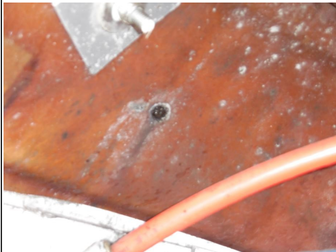
Swim Platform Bolt - Signs of Corrosion
